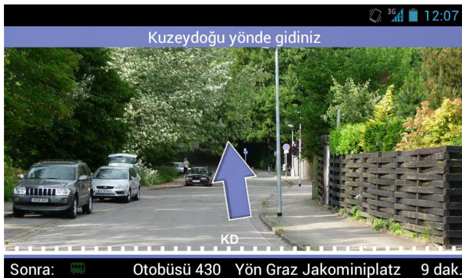
Figure 18: Augmented reality navigation with navigation instruction, heading and info about the next destination
