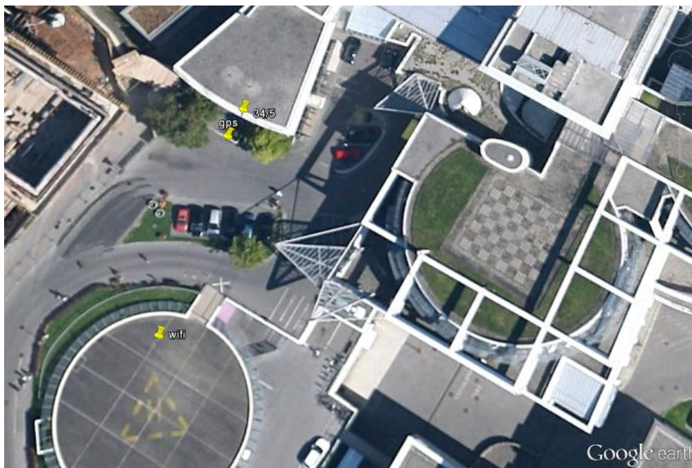
Figure 9: Measurement result for reference point 34/5 (Kinderklinik). The GPS fix for that position was within 5 meters accuracy. The positioning fix obtained by wifi deviated 35 meters.
