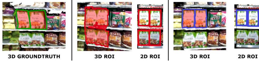
Figure 5. Automated ROI detection in the 2D and 3D domain. (left) 3D ground truth annotation. (mid) ROIs computed in 3D out of automatic 2D detections. (right) 3D ROIs computed out of the 2D ground truth data.
