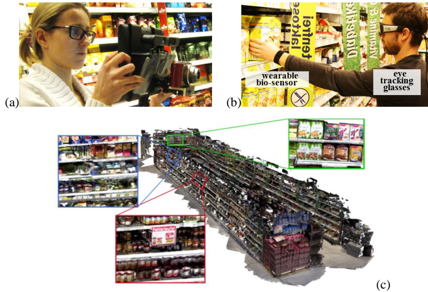
Figure 3. Hardware (a) for the 3D model building process (Kinect and HD camera), (b) study with packages, (c) 3D model of the study environment, a shop floor for experimental studies.
