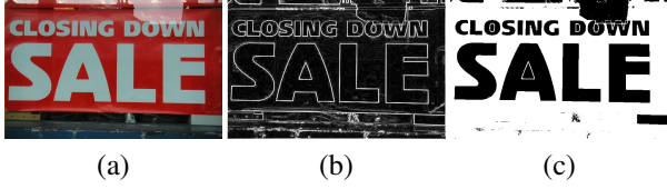
Figure 3. Intensity gradient magnitude channel \nabla . (a) Source image. (b) Projection output. (c) Extremal Regions at threshold \theta = 24 (ERs bigger than 30% of the image area excluded for better visualization)
